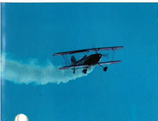
Above: Crop dusting coverage can be easily assessed when GTE phosphors are added to agricultural chemicals.
